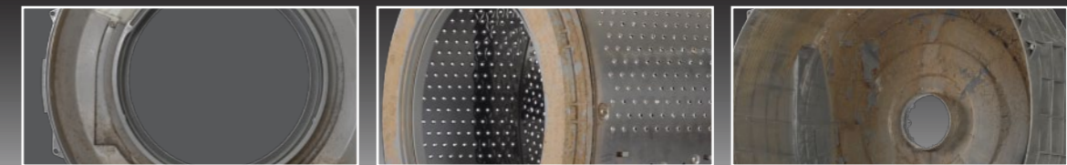
Dirt behind the front cover of the outer tub Dirt on the front of the stainless steel tub Dirt on the inside of the outer tub
